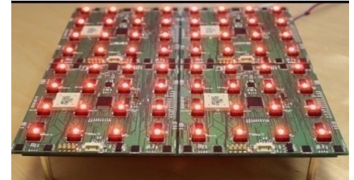
Tiles composing the first version of the tabletop (source: RFIdées company)
